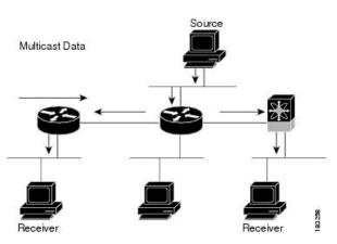
Figure 1: Multicast Traffic from One Source to Two Receivers
