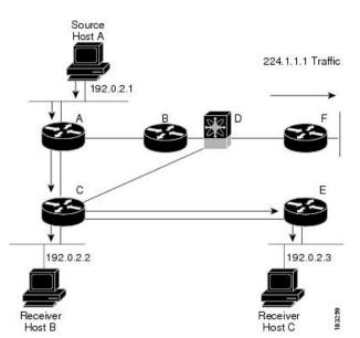
The notation (S, G) represents the multicast traffic from source S on group G. The SPT in this figure is written (192.0.2.1, 224.1.1.1). Multiple sources can be transmitting on the same group.
