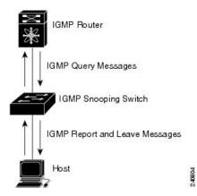
The IGMP snooping software operates upon IGMPv1, IGMPv2, and IGMPv3 control plane packets where Layer 3 control plane packets are intercepted and influence the Layer 2 forwarding behavior.
