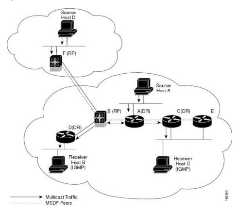
Figure 6: PIM Domains in an IPv4 Network
