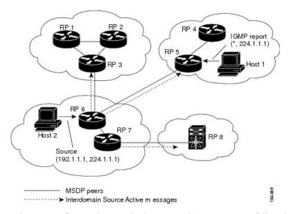
When you configure MSDP peering between each RP, you create a full mesh. Full MSDP meshing is typically done within an autonomous system, as shown between RPs 1, 2, and 3, but not across autonomous systems. You use BGP to do a loop suppression and MSDP peer-RPF to suppress looping SA messages.
