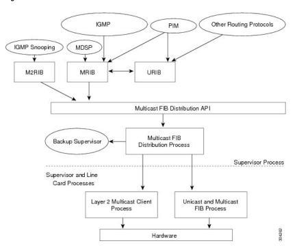
Figure 7: NX-OS Multicast Software Architecture
