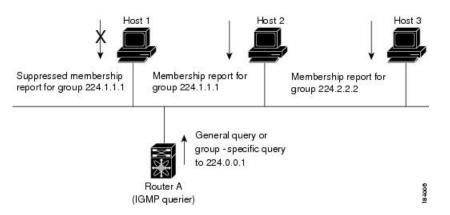
In the figure below, router A, which is the IGMP designated querier on the subnet, sends query messages to the all-hosts multicast group at 224.0.0.1 periodically to discover whether any hosts want to receive multicast data. You can configure the group membership timeout value that the router uses to determine that no members of a group or source exist on the subnet.
