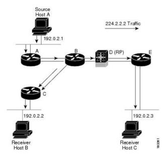
The notation (\*, G) represents the multicast traffic from any source on group G. The bidirectional tree in the figure is written as (\*, 224.2.2.2).
